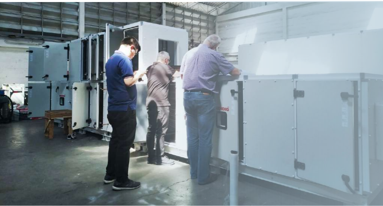
Above: Eurovent Expert team was inspecting H-PTP according to RS of HAHU in Thailand 2019. The detailing design of unit such as maximum gap between panel and structure frame -works, opening access for service, material corrossivity report were evaluated and certified H-PTP-range.
