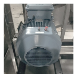
Explosion proof motor and or IE-1.2. and 3 as per optional for MTP-Fan configuration
