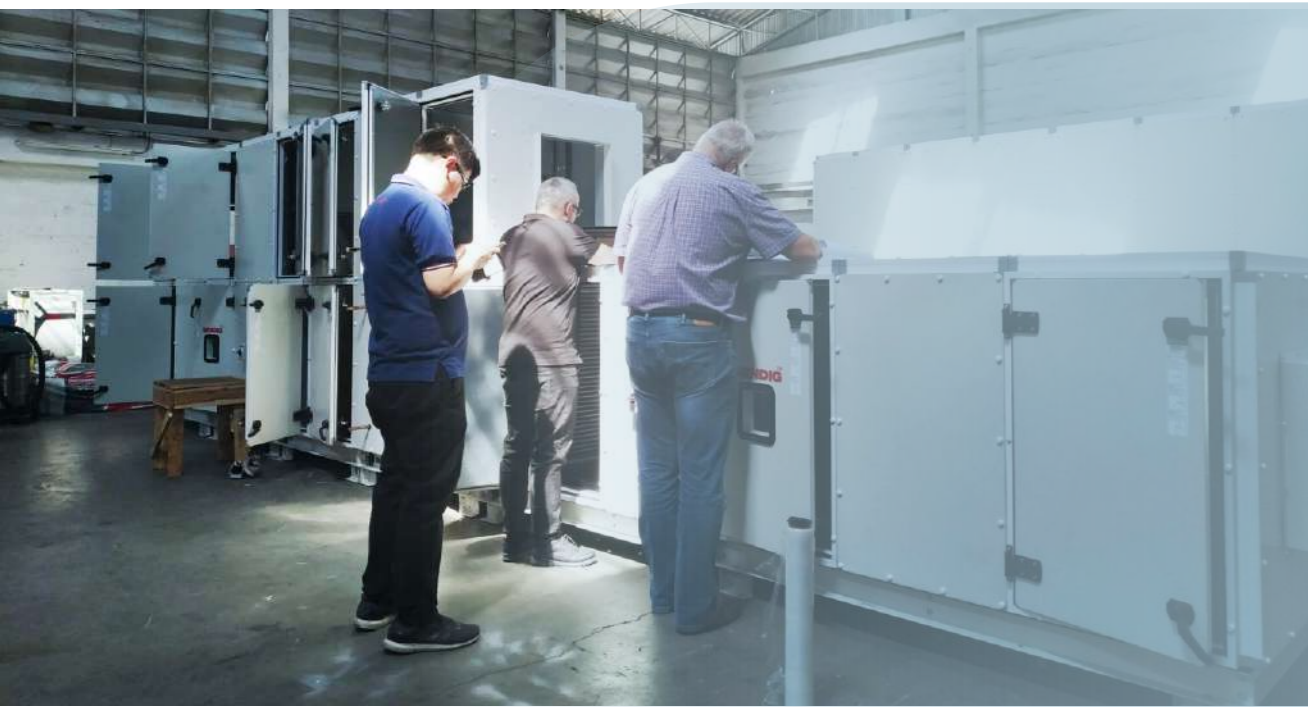
Above: Eurovent Expert team was inspecting PTP-H according to RS of HAHU in Thailand 2019. The detailing design of unit such as maximum gap between panel and structure frame -works, opening access for service, material corrossivity report were evaluated and certified PTP-H range.
